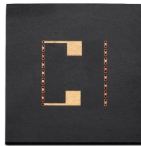
Fig.13: Laser direct-structured through-hole plating (rear side) of a daisy-chain AMR sensor
