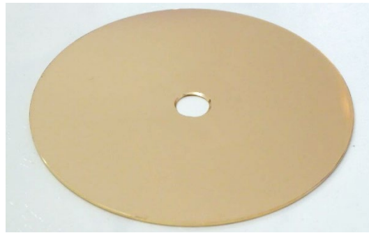
Fig. 8: Wafer coated with gold PVD (cathode sputtering)
