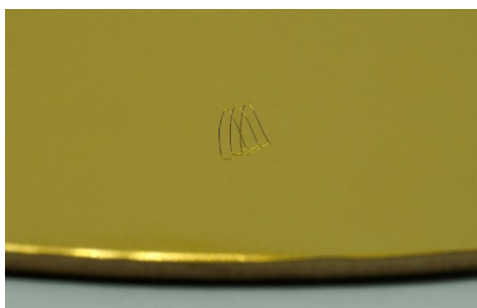
Fig. 20: Thin wire bonds on 200 nm Au (PVD) on TECAWAFER PEEK LDS black
