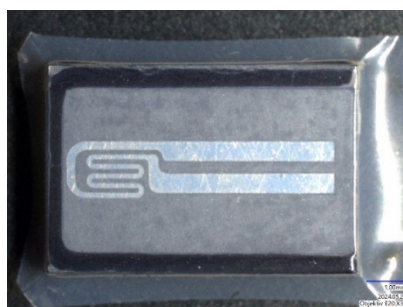
Fig. 19: PEEK foil welded onto temperature sensor
