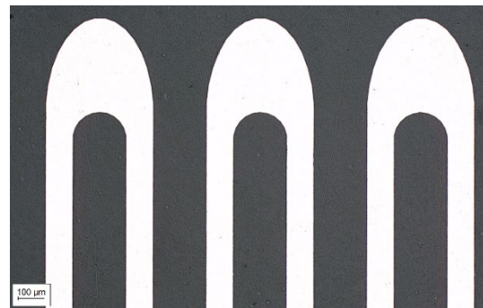
Fig. 10: Lithographically structured and PVD-coated wafer (100 nm NiFe)
